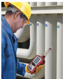
Multi RAE Benzene used for leak detection
