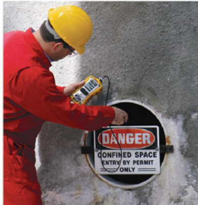
Confined space testing with the MultiRAE Lite
